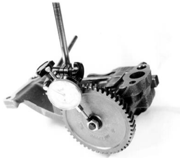
Checking Pump Shaft Side Movement
