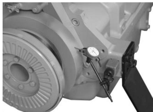
Measuring Runout of Dual Damper
