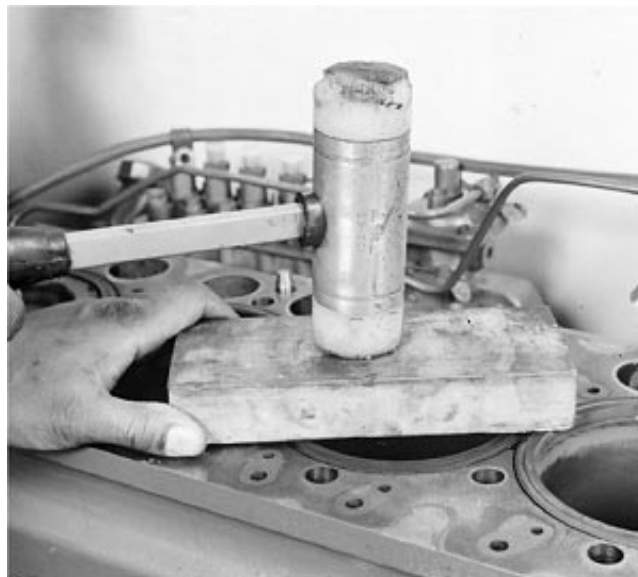
Seating Cylinder Liners in Block
