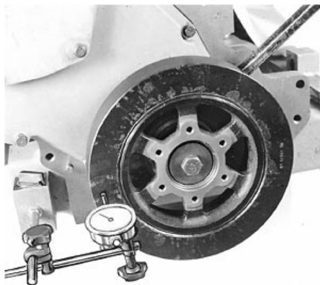
Checking Crankshaft End Play
