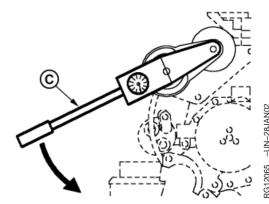
Align Torque Wrench With Pulley And Tensioner
