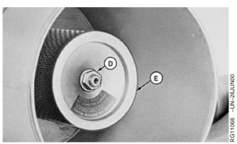
Retaining Nut and Secondary Element
