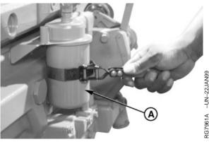
Removing Oil Filter Element
