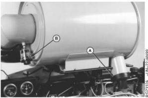
Dust Unloader Valve and Indicator Gauge
