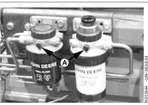
Air Bleed Vent Screws (Dual Filter Option Shown)
