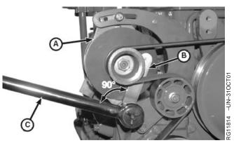
Belt Tension Tool and Torque Wrench
