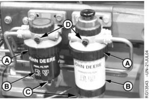
Dual Fuel Filters (Primary Filter with Bowl at Left, Final Filter at Right)
