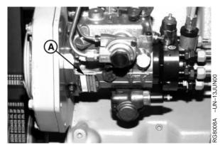
Record Injection Pump Serial Number
