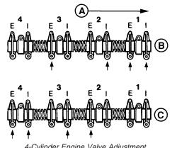
4-Cylinder Engine Valve Adjustment
