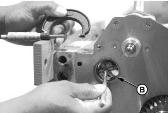
Balancer Shaft Bore ID (Bushing Installed)
