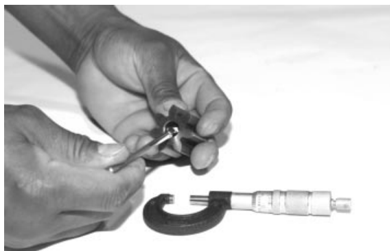
Measure Idler Gear ID for Wear
