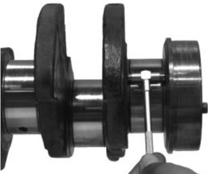
Measuring Main Thrust Journal Width
