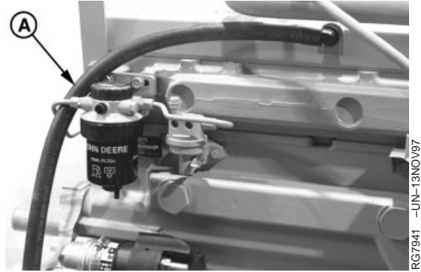
Ventilator Outlet Hose Inspection
