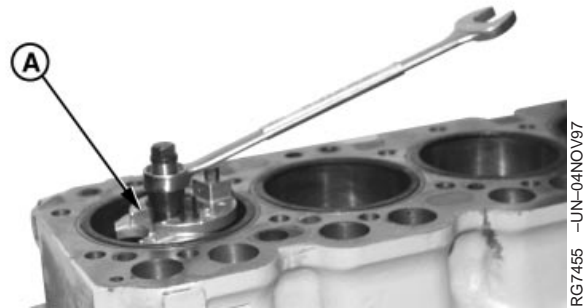
Using Ridge Reamer in Cylinder Bore
