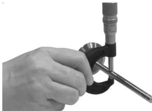
Valve Stem Measurement
