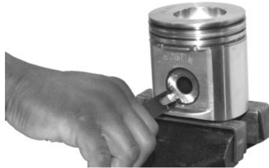
Piston Pin Snap Ring Removal
