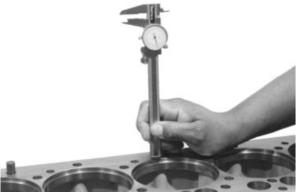
Measure Liner Flange Counterbore Depth
