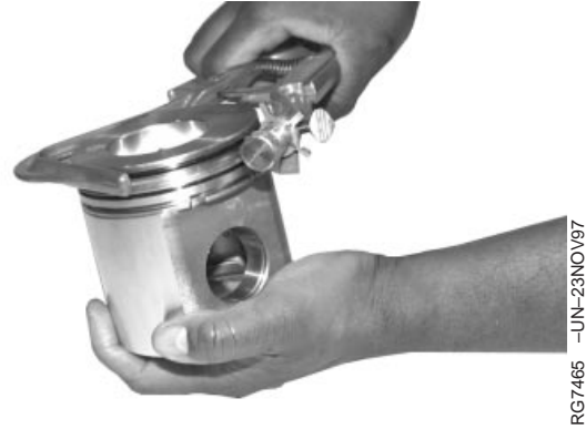
Cleaning Piston Ring Grooves
