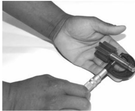
Measuring Drive Shaft OD for Wear
