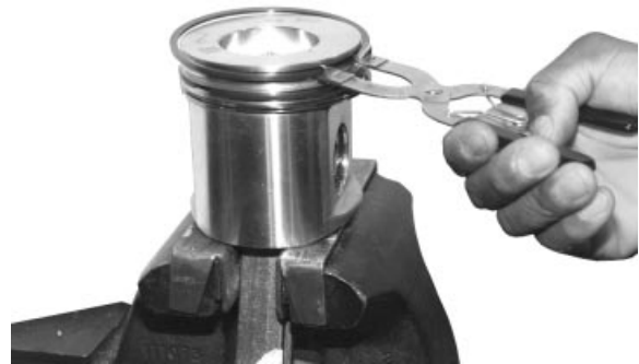
Piston Ring Removal from Piston
