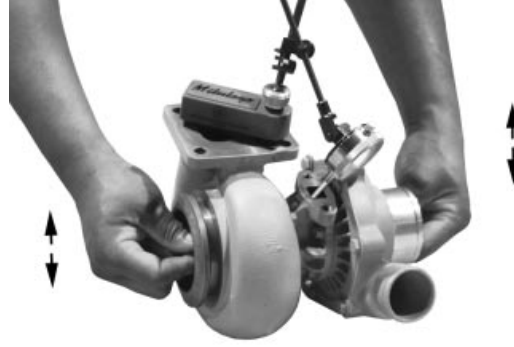
Radial Bearing Clearance Test
