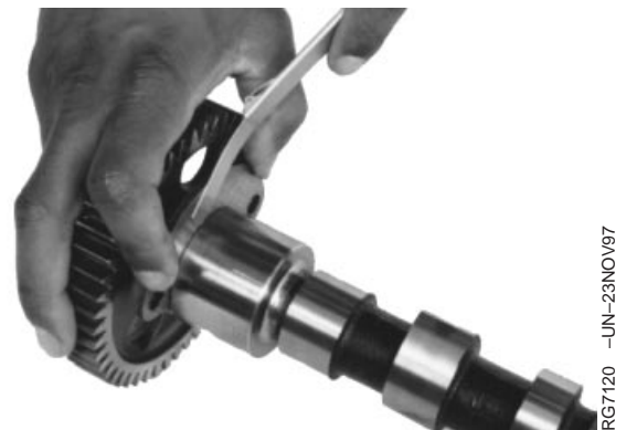
Measuring Camshaft Thrust Plate
