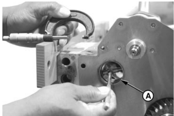
Measuring Balancer Shaft Bushing ID
