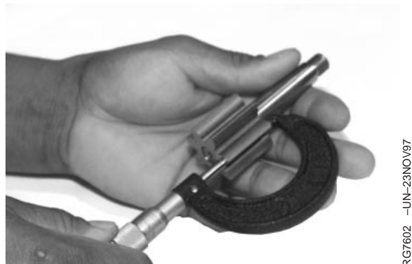
Checking Gear Thickness
