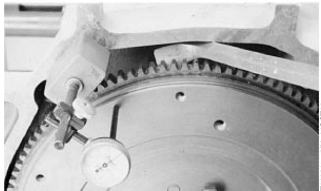
Check Crankshaft End Play w/Dial Indicator
