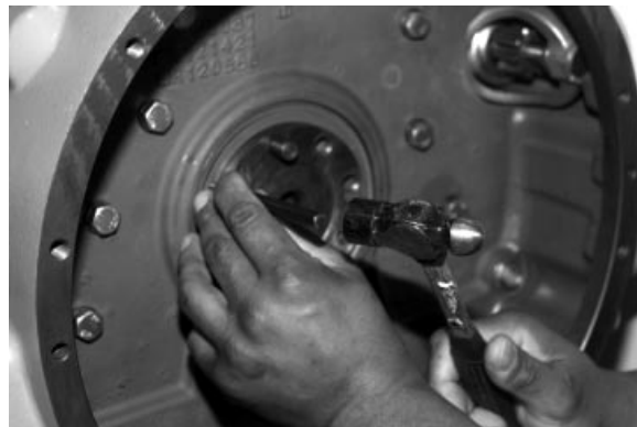
Setting Puller Removal Screws
