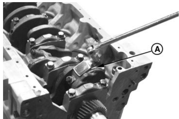
Bearing and Rod Cap Removal
