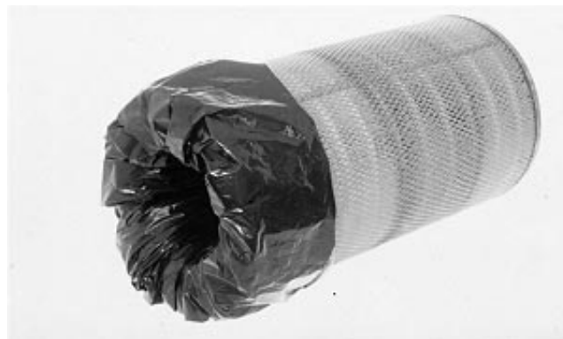
Air Intake Leak Test
