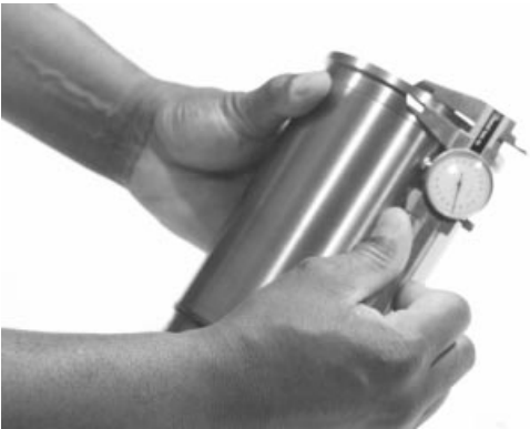
Measuring Liner Flange Thickness
