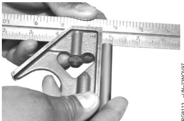
Push Rod End Crown Wear
