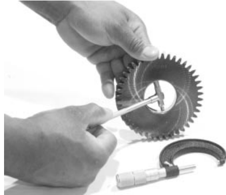
Measuring Idler Gear Bushing ID
