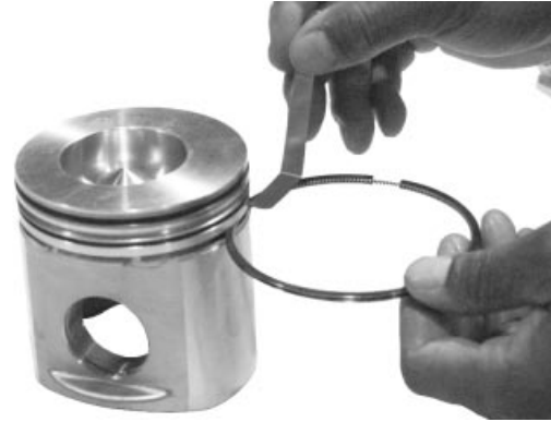
Piston Ring Groove Wear
