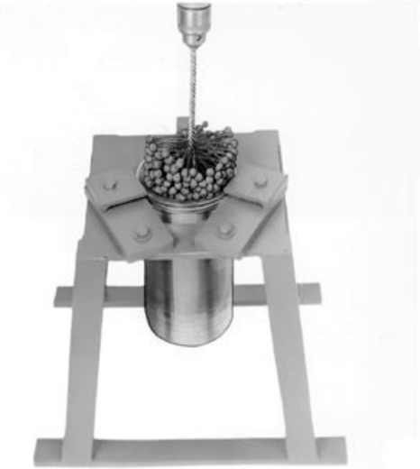
Cylinder Liner Deglazing
