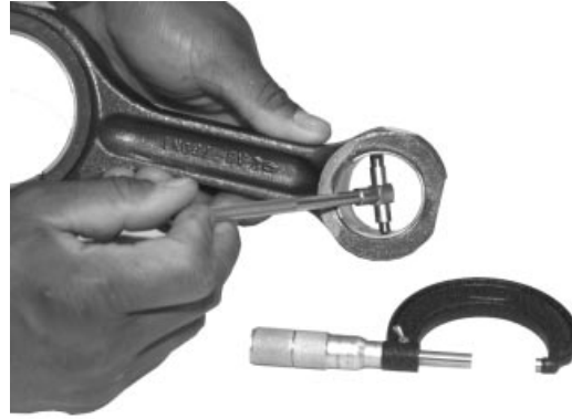
Measuring Connect Rod Pin Bore ID
