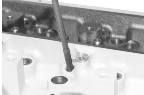
Fuel Injection Nozzle Bore Cleaning
