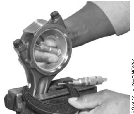
Measuring Rod Bearing ID
