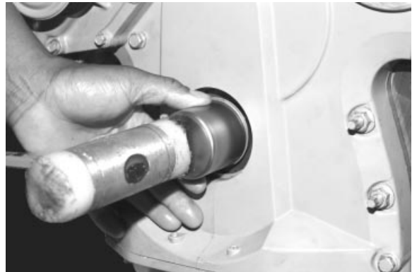
Installing Crankshaft Wear Sleeve
