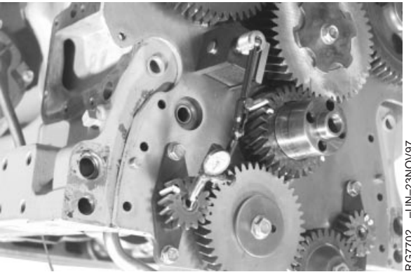
Measuring Balancer Shaft End Play—4-Cylinder
