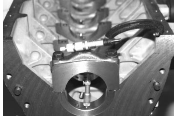
Measuring Assembled Main Bearing Cap ID
