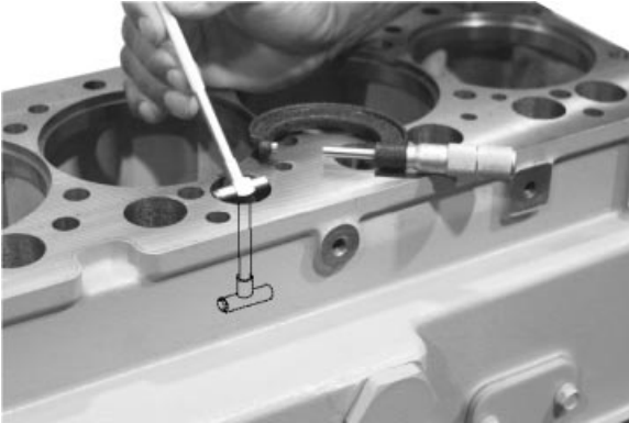
Measuring Camshaft Follower Bore
