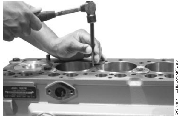
Marking Cylinder Liner Location/Position
