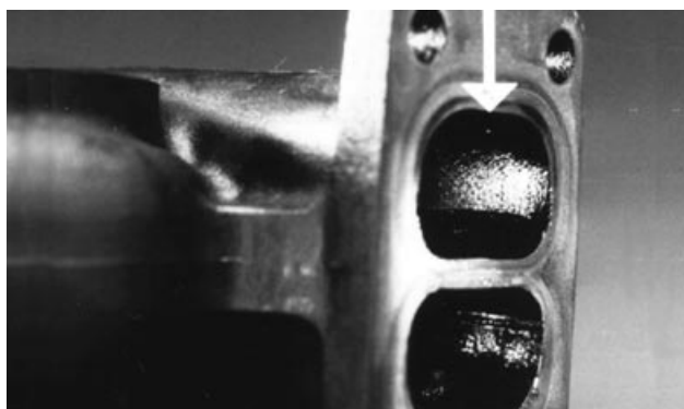
Checking Turbine Housing Inlet Ports
