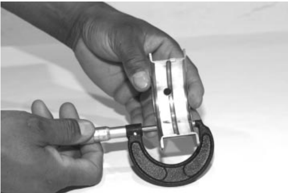
Measuring Main Thrust Bearing Width
