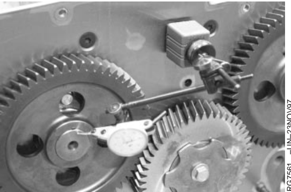
Measuring Camshaft End Play
