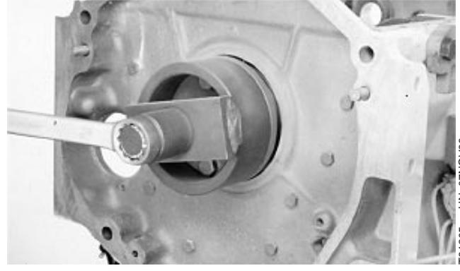
1. Position the guide plate from JT30040B or KCD10002A tool over dowel with two cap screws. Finger tighten both cap screws until they contact the pilot.
