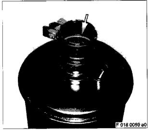
Coat O-ring (arrow) with denaturated ethanol. Insert sleeve, see next illustration.
