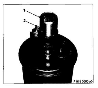
Insert sleeve (1) and tighten with hex screw (2).
