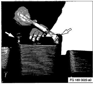
Before installing, coat O-rings (arrow) with petroleum jelly.
