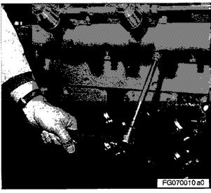
Tighten hex screws for connectors to crankcase to specified tightening torque – see Overview drawing C 077.05.01.
