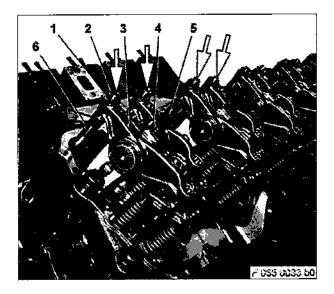
Fit valve bridge(s) in accordance with marking (installation location) on sliding pin in cylinder head.
