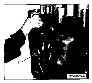
Press off thermostat housing (1) from coolant distribution housing.
