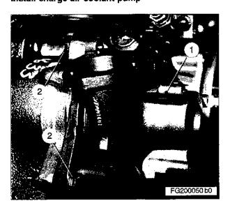
Coat O-ring with petroleum jelly (see Overview drawing C 203.05.01) with petroleum jelly and insert in groove on pump housing of charge air coolant pump.
