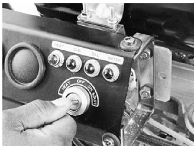
Starting Engine Using Key Switch (Earlier Engines)
