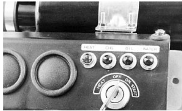
Key Switch in "ON" Position (4.5 L "270" Engines)
