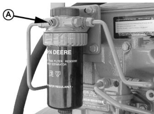
Final Fuel Filter Bleed Vent Screw
