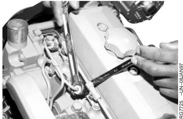
Bleed At Fuel Injection Nozzles
