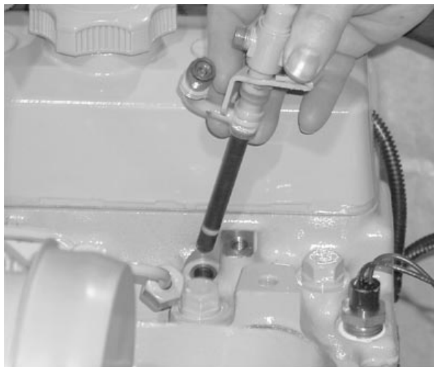
Injection Nozzle in Cylinder Head
