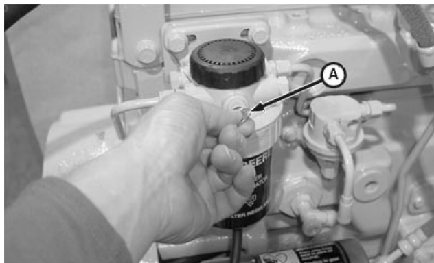
Final Fuel Filter Bleed Vent Screw
