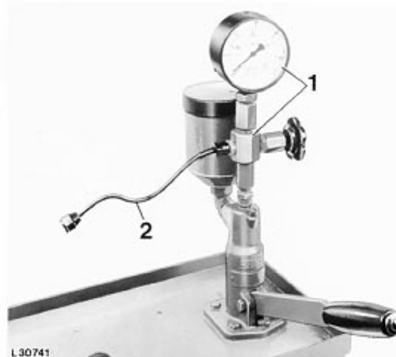
Fuel Injection Nozzle Test
