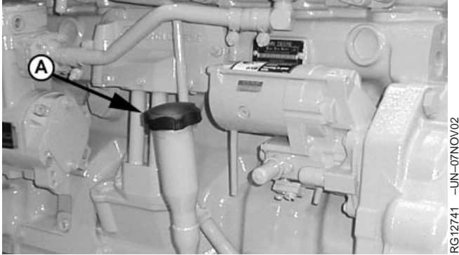
Check Engine Oil Level (Left-Side Option Shown)
