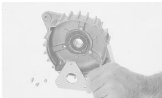
Install Bearing Retainer
