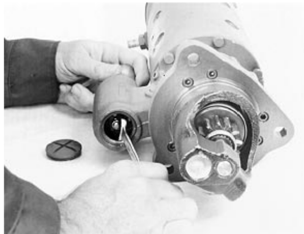
Remove Commutator End Frame
