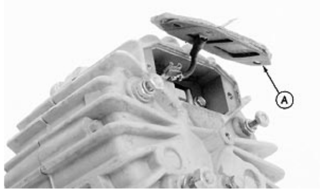
Remove Brush Cover and Gasket
