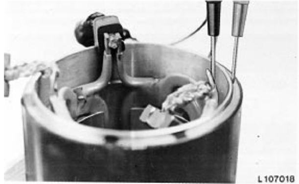
Test Field Winding for Grounded Circuits
