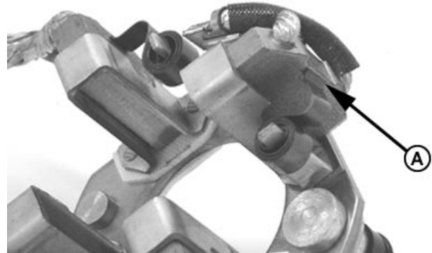
Measure Brush Spring Tension
