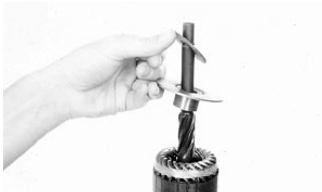
Lubricate Splines and Armature Shaft
