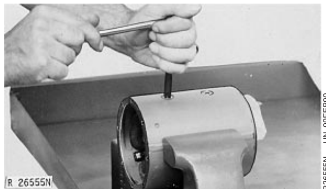
Remove Field Windings
