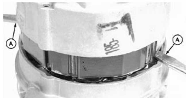
Insert Screwdriver Blades
