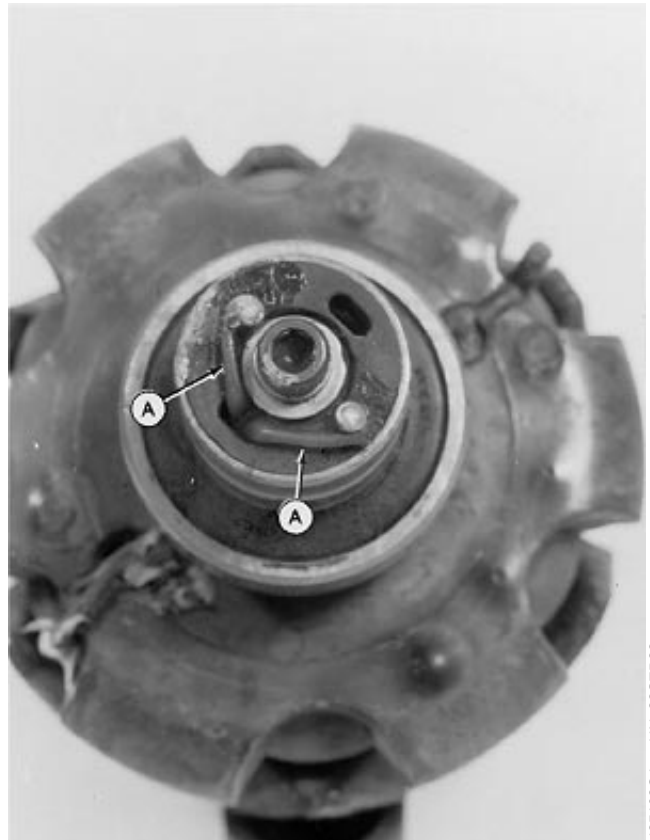
Wrap Leads Around Terminals
