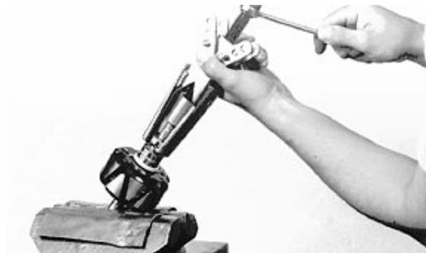
Remove Rear Bearing
