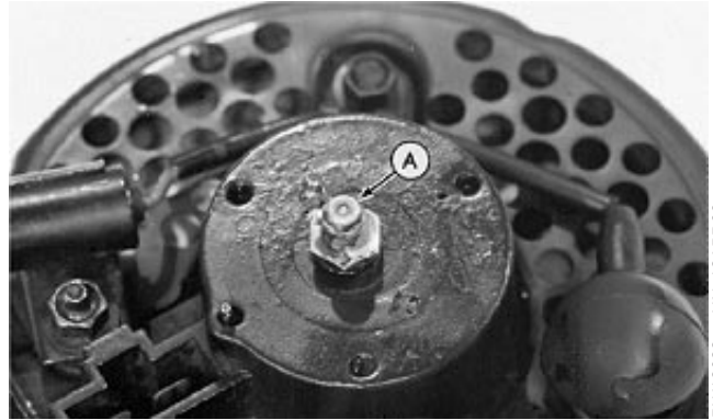
1/16-27 NPT Grease Zerk
