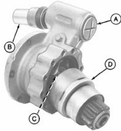
Solenoid Plunger/Shift Lever Assembly
