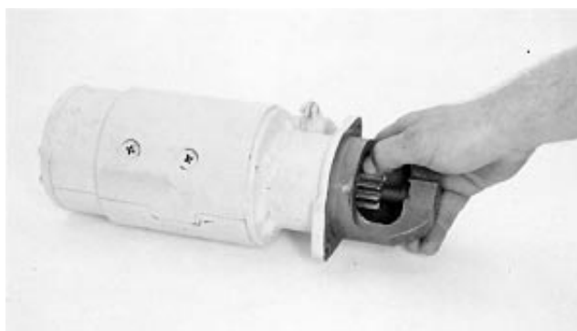
Turn Overrunning Clutch Pinion
