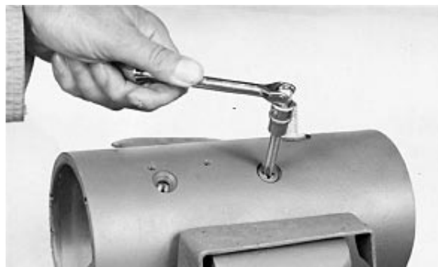
Remove Field Windings
