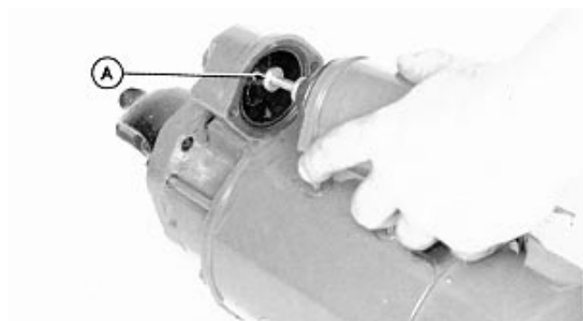
Solenoid Plunger Shaft
