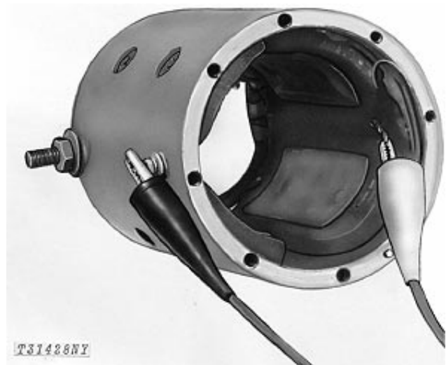
Make Open Circuit Test for Shunt Windings
