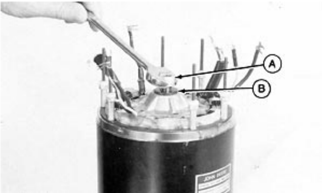
Hardened Washer and Nut
