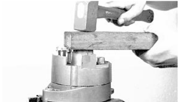
Install Rear Housing
