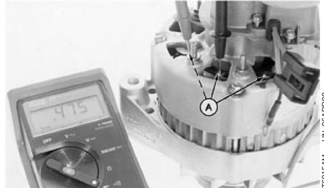
Test Positive Diodes
