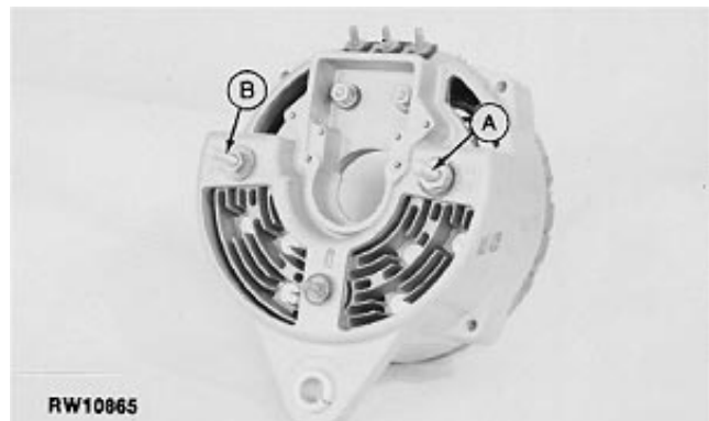
Remove Diode Heat Sink Assembly
