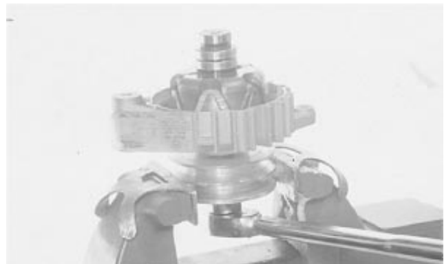
Install Rotor to Housing
