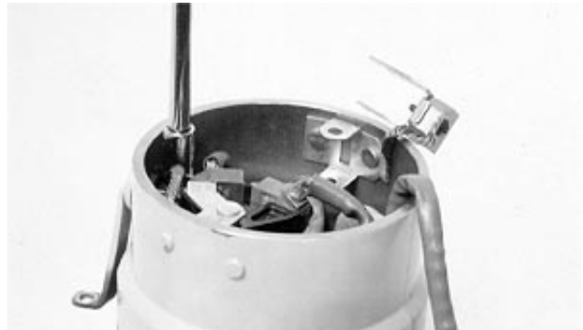
Remove Field Connector
