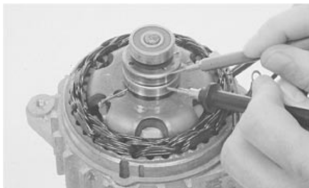
Check Rotor Windings
