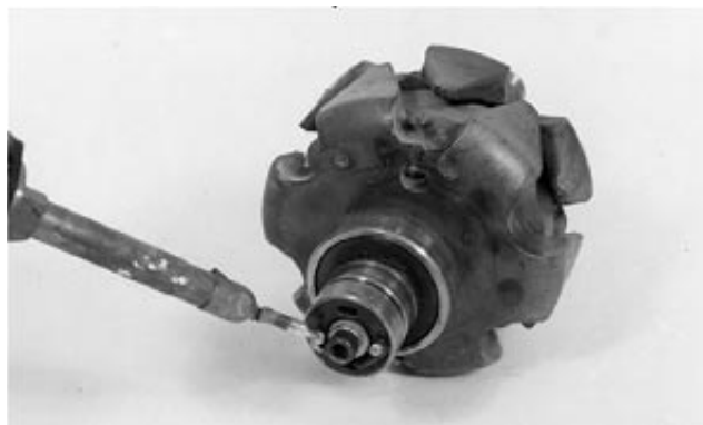
Inspect Rotor Shaft and Body
