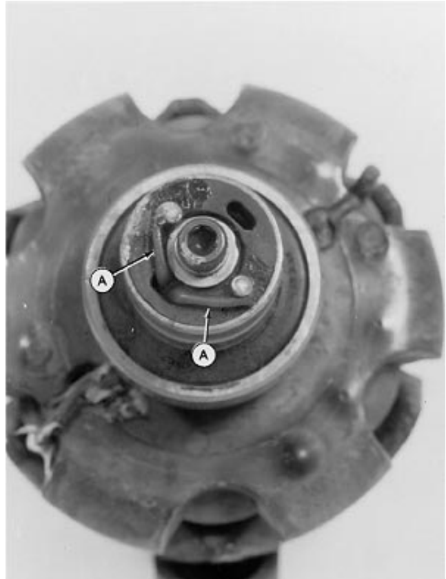
Wrap Leads around Slip Ring Terminals
