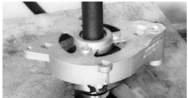
Press Front Housing onto Rotor Shaft
