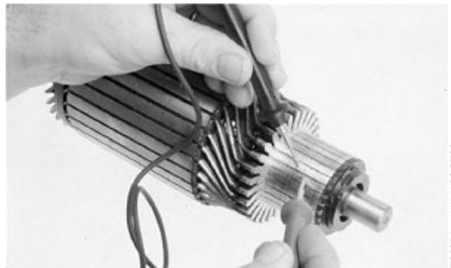
Make Open Circuit Test
