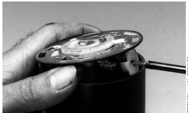
Remove the Disassembly Sleeve
