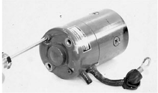
Remove Cap from Frame Assembly
