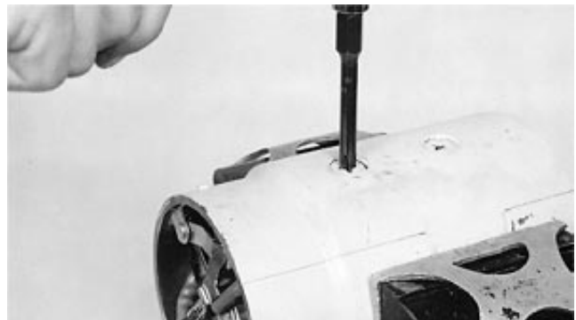
Remove Field Windings
