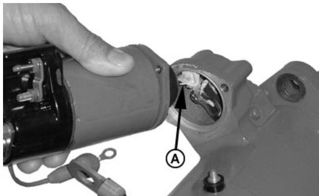
Lift Plunger Shaft
