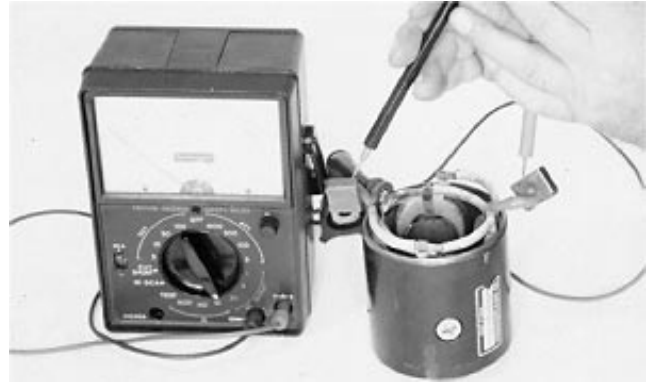
Check for Open Field Coil
