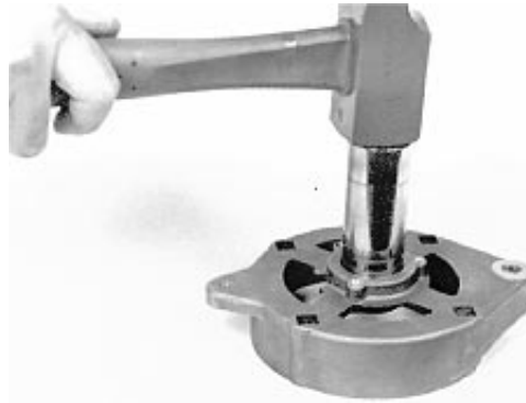
Extract the Front Bearing
