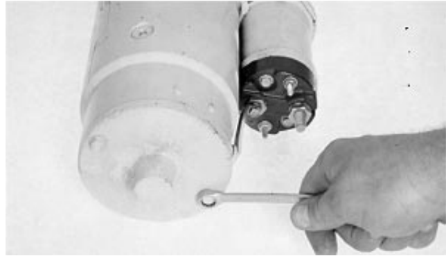
Install Commutator End Frame
