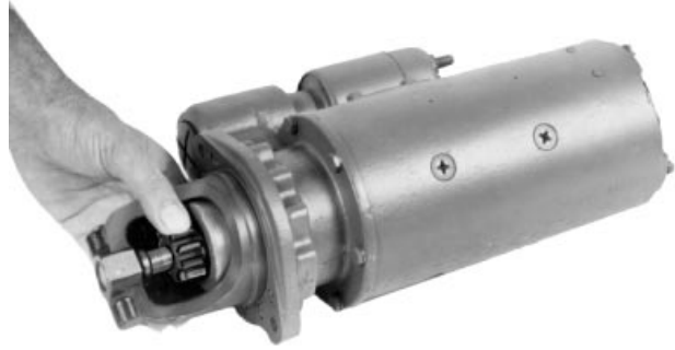
Turn Overrunning Clutch Pinion
