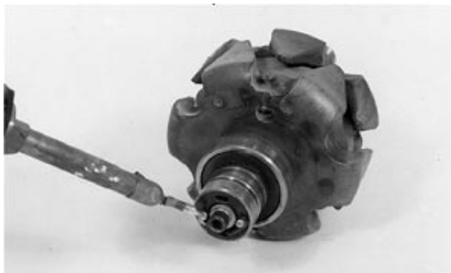
Unsolder Rotor Leads
