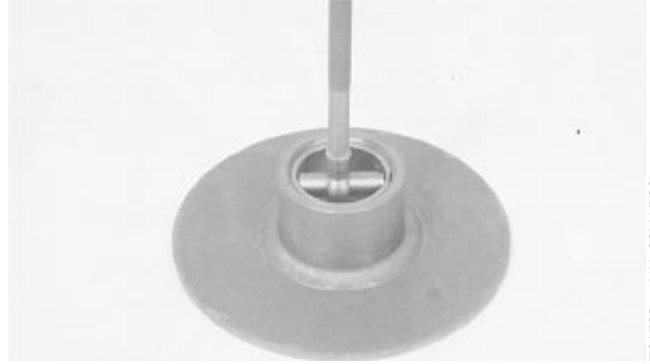
Inspect Center Bushing ID
