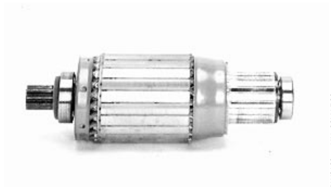
Inspect and Repair Armature
