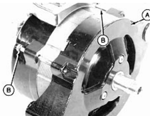
Secure Front Housing
