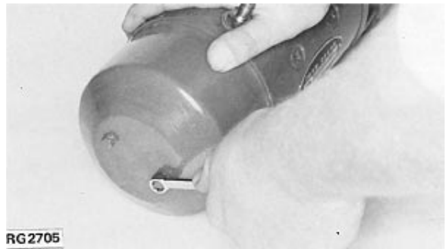
Remove End Frame Cover and Gasket
