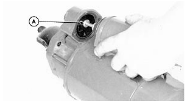
Lift Plunger Shaft
