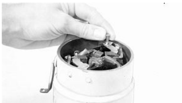
Remove Pins, Holders, and Springs
