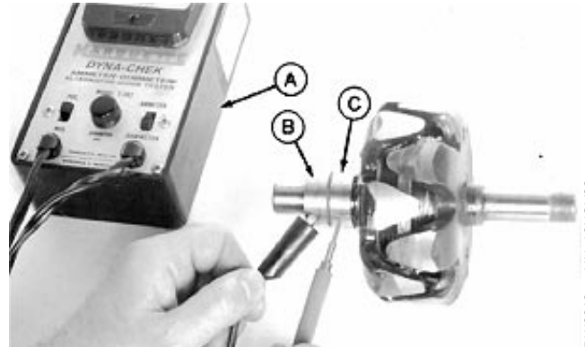
Test Rotor for Open Circuit
