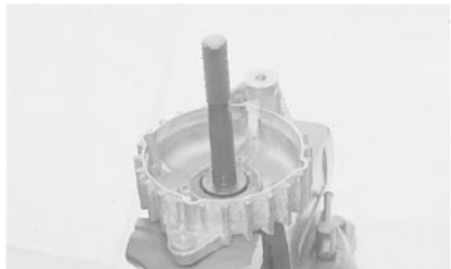
Install Seal in Housing Bore
