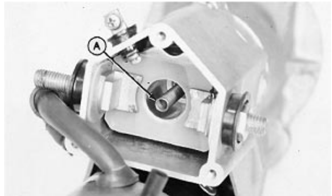
Remove Plunger Spring
