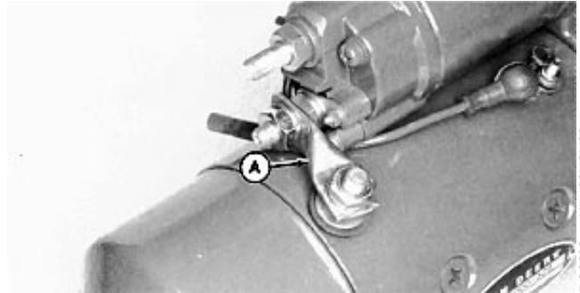
Remove Field Coil Connector
