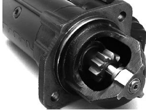
Check Overrunning Clutch Pinion
