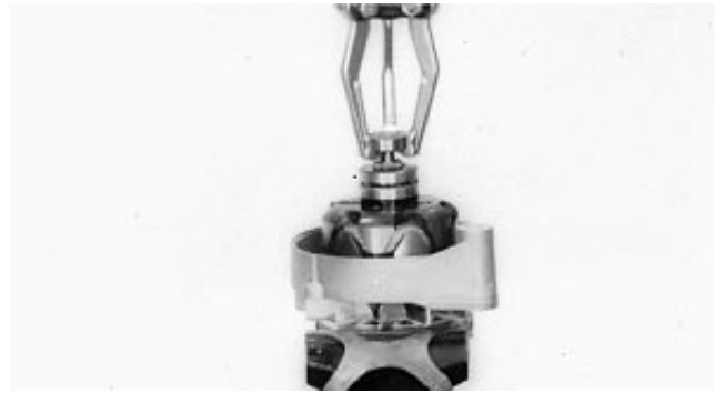
Remove Slip Ring End Bearing
