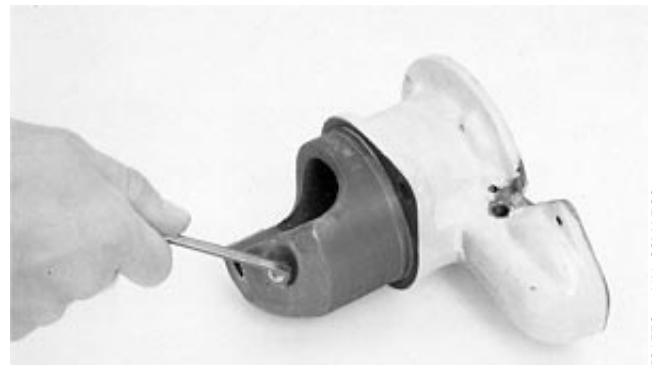
Remove Plug and Drive End Wick
