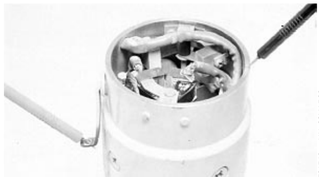
Make Ground Circuit Test
