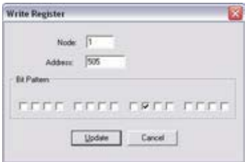
Fig. 218: Power factor setpoint
