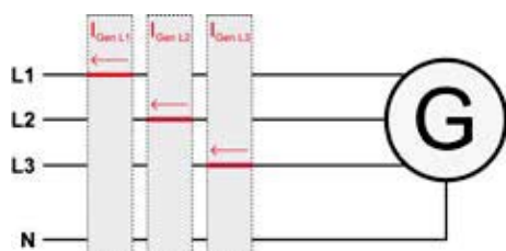
Fig. 46: Current measuring - generator, L1 L2 L3
