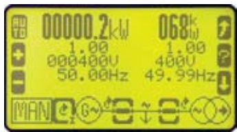
Fig. 129: Setpoints screen (MANUAL operating mode)
